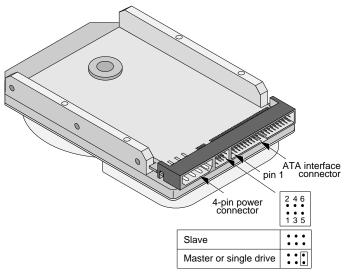
Figure 1. Master and slave jumper settings
