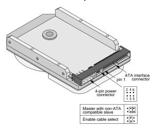
Figure 5. Non-ATA compatible and cable select jumpers Non-ATA compatible slave jumper
