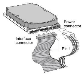
Figure 4. Cable connectors
