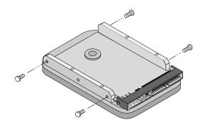
Figure 3. Mounting screws
